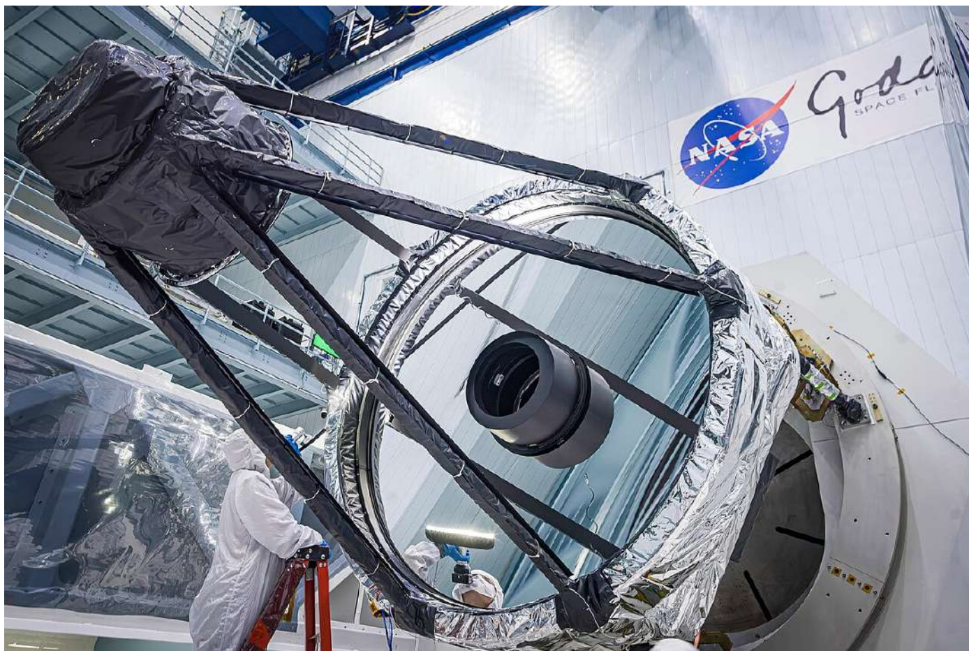
The primary mirror of the Roman Space Telescope; donated to NASA by the NRO in 2012. Credit: NASA/Chris Gunn
